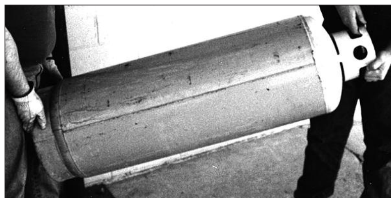
Photo 5: This is the proper way to carry a 100-pound cylinder.
