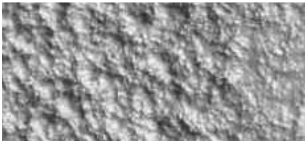
Photo 3: Coarse orange peel surface texture
