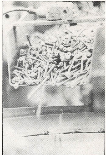
Tapdek blanks, with heads formed, drop into a point-forming machine.
