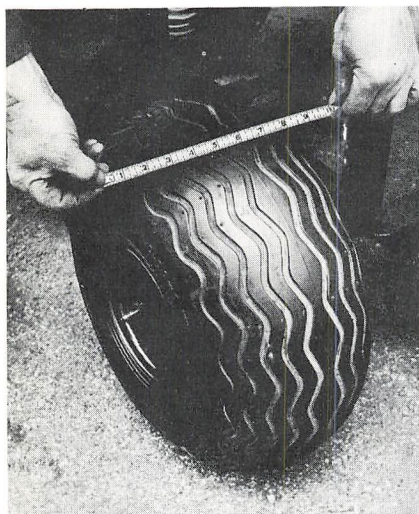
Extra big balloon tires protect roof by greater distribution of weight.
