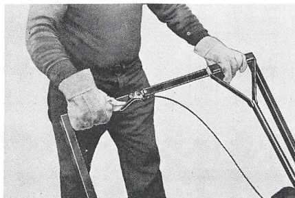
Dead Man Safety Feature, when operator lets go, machine comes automatically to a stop.
