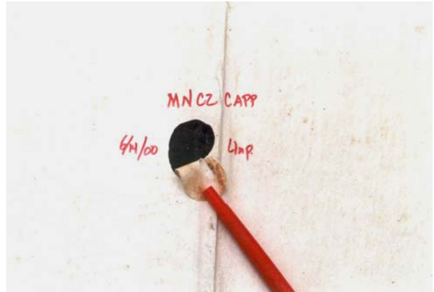
Photo 14: White acrylic coating applied to an asphalt-based membrane, that lacks asphalt emulsion primer, revealed less bond and peel strength. Note only minor traces of asphalt residue on the bottom side of acrylic coating.
